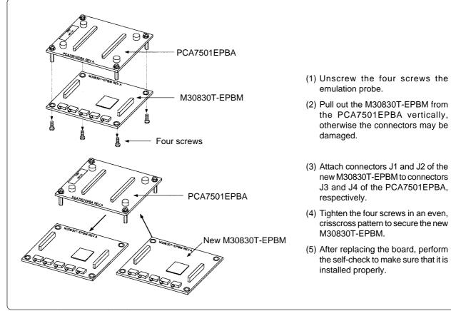
Figure 1 Replacing MCU boards
